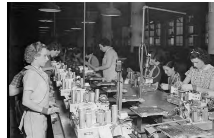
Camden, New Jersey – Radio. RCA Victor. End of Chassis assembly line – assembling 5-tube radio chassis (1937).
